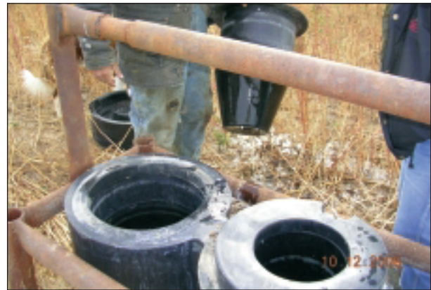
A view of the tapered bowl when it is removed from the cylinder
