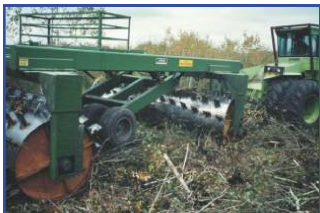
Roller chopper consists of two offset drums with angled steel paddles. It weighs 28,000 lbs empty & 58,000 with water. Photo: Ron Moss
