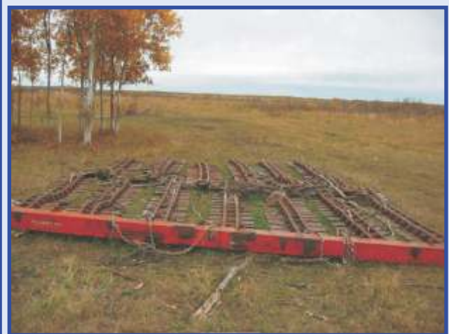
Bark scraper made out of used bulldozer tracks. Photo: Ron Moss
