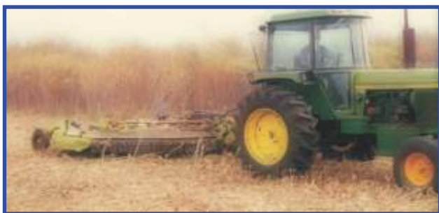
Pull-type brush mowers are used to control woody growth up to 2 inches (5 cm) in diameter.
